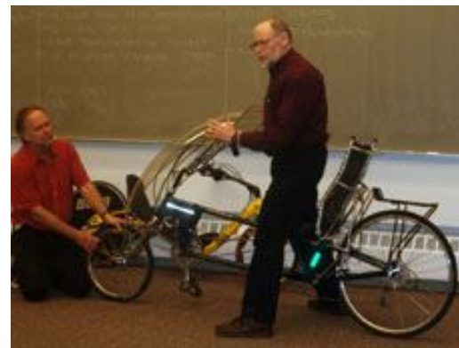
BILL FREY showed his Tour Easy Fold Rush that he bought last year. The rear swing arm has an elastomer to provide limited suspension. Removing a pin enables the swing arm, with wheel attached, to be folded under for compact storage and transportation. Bill's bike also has the optional Pantour suspension front hub.
