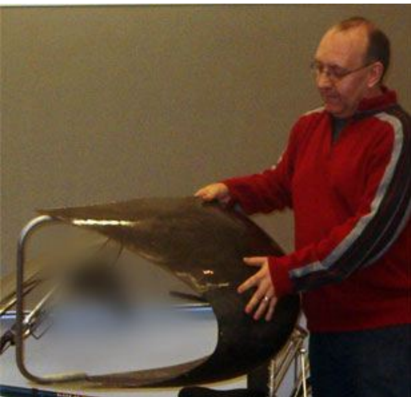
RICK WIANECKI of Okemos shows the nose cone for his latest project, a velomobile (pedal car), an enclosed three-wheeler that will lean when cornering.
