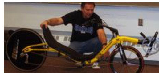
DON SMITH of Sterling Heights talked about the latest changes he's made to his Optima Baron, which bring the weight down to only 18 pounds, 8-1/4 ounces. The front wheel has only 10 spokes and is intended for racing wheelchairs. The carbon fiber Renn back wheel is a solid disk, with no dish.
