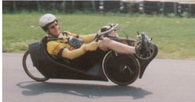
DAVID BALFOUR of Marietta, Ill., raced his award-winning homebuilt carbon fiber low racer to third place in the streamliner class. The worst he finished in any single event was fifth in the coast-down.
