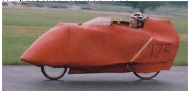
RICH SADDLER of Quakertown, Pa., finished second in the super street class in his homebuilt streamliner with foam fairing.
