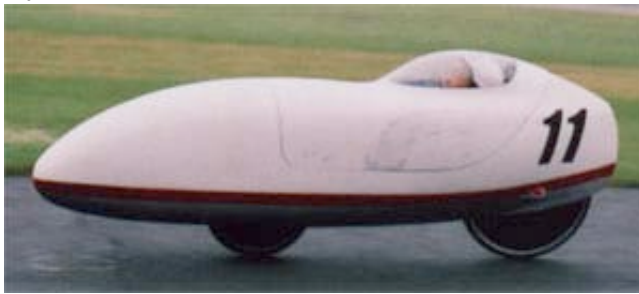
SINCE RACING his front-wheel-drive Varna clone at the 2004 rally, Kevin Berls of Sunbury, Ohio, made changes including lowering the seat so his head wouldn't bump on the canopy and replacing the original tiller steering with a remote system. Garrie Hill made the monocoque lower part of the fairing and the two top pieces; Kevin did the rest. Despite the improvements since last year, he said, "You got to work to ride it." (Charles Brown photo)
