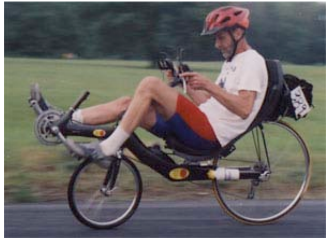
JIM IWASKOW of Richmond Hill, Ontario, raced his homebuilt carbon fiber bike. He's ridden it about 10,000 km since building it in 2002. He made the frame by laying carbon fiber over a foam mold. The handlebars and seat also are carbon fiber. He's now building another carbon fiber bike, with front and rear suspension.
